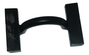
The double roofing seamer is used to shape the standing seam.
